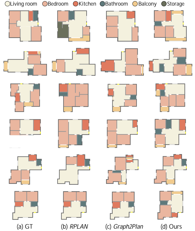
Fig. 10. Comparison to the state-of-the-arts with the only boundary constraint. Each row shows the results of different methods applied to the same boundary. (a) The ground truth floorplans, and the floorplans generated by (b) RPLAN , (c) Graph2Plan and (d) our method.
