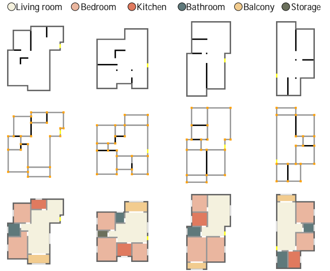
Fig. 12. Loading-bearing wall constrained generation. Top row: the input boundary as well as the loading-bearing walls. Middle row: the generated wall graphs with the loading-bearing walls (in black) using our method. Bottom row: the corresponding floorplans for visualization.
